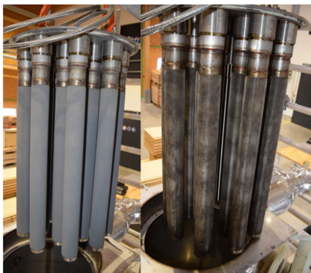
Fig. 8 Metal mesh filter before and after cleaning
