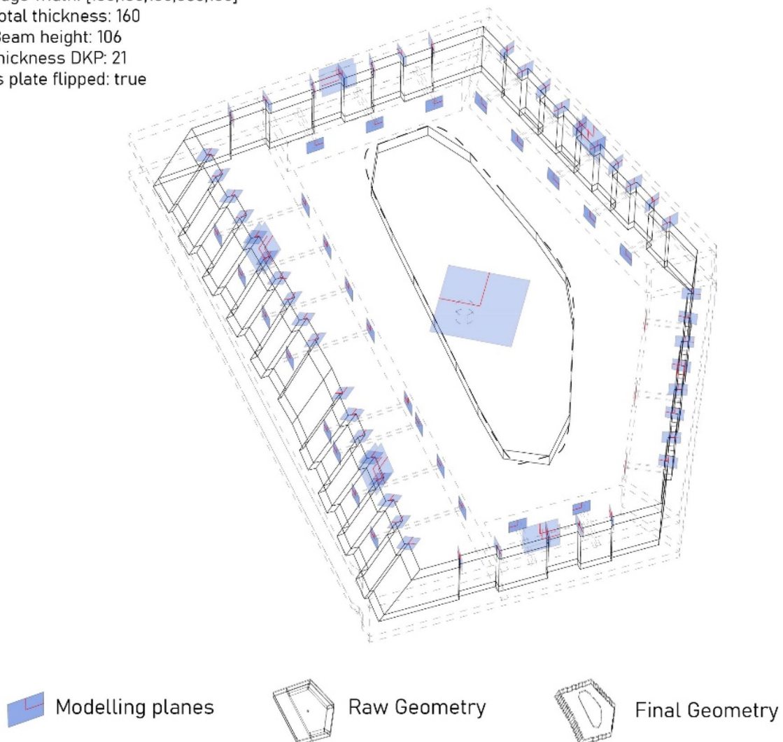
Fig. 7 Exemplary computed geometry and data as stored in the cassette data file. It forms the base input for the robotic milling of cassettes, including raw mesh for simulation visualization and frames and curve objects for accurate fabrication routine generation
