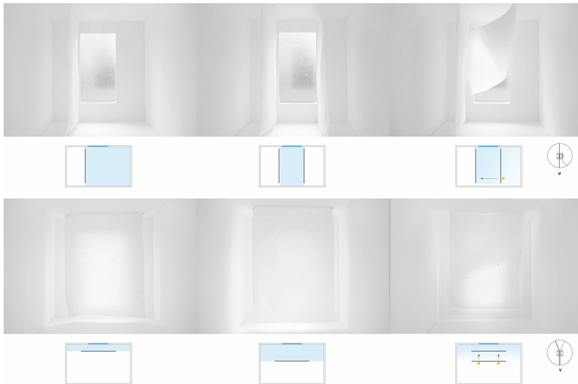
Fig. 7 Light studies. The blue area shows which areas receive direct light. Model 1:10
