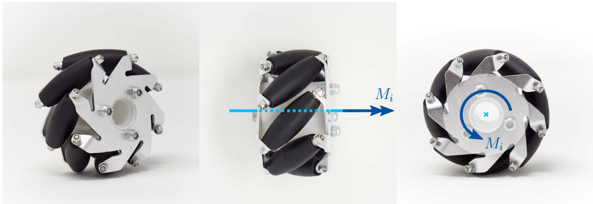
Figure 4.3: Different perspectives of a Mecanum wheel as used on the custom mobile robot
