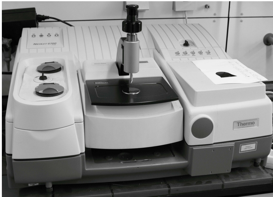
Abb. 2.17: FT-IR-Photospektrometer Nicolett 6700 Research (Fa. Thermo Fisher Scientific, Waltham, MA, USA).
