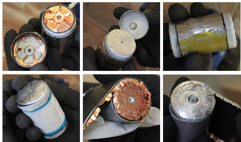
Figure 8. Opening the 4680 battery cell.
