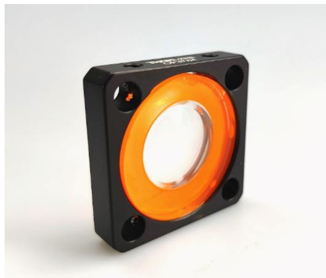
Figure 11. The orange-dyed adhesive spreads well on the surface provided for bonding, leaving out the microstructured surface in the middle of the lens.
