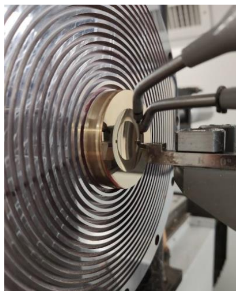
Figure 3. Turning of the brass master with optical surface finish.
