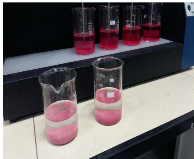
Fig. 109 Removal of RR 195 with charred dolomite by stirring the suspension in a Jar Tester
