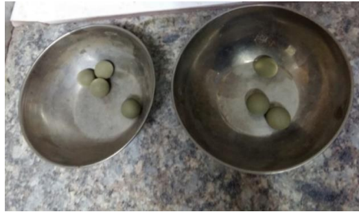
Fig. 37 Green granules made of the spent adsorbent, water and additive (quality control laboratory at LECA CO.) (photo: E. Khalilzadeh Shirazi)
