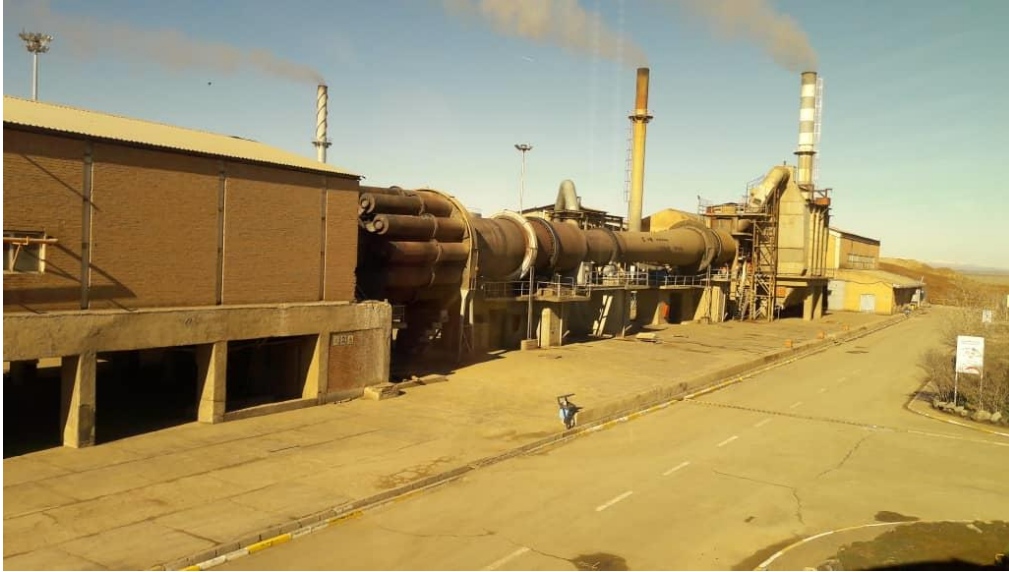
Fig. 40 Installations for heat treatment of the green granules in different phases of drying, burning and cooling at the LECA CO. (photo: E. Khalilzadeh Shirazi)
