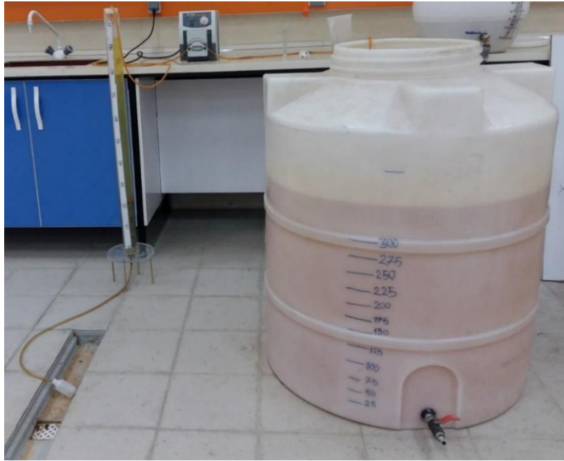
Fig. 35 Treatment of acrylic fiber dyeing wastewater using natural granular bentonite in a fixed-bed continuous system (Laboratory of Water and Wastewater Treatment at Azad University in Iran)
