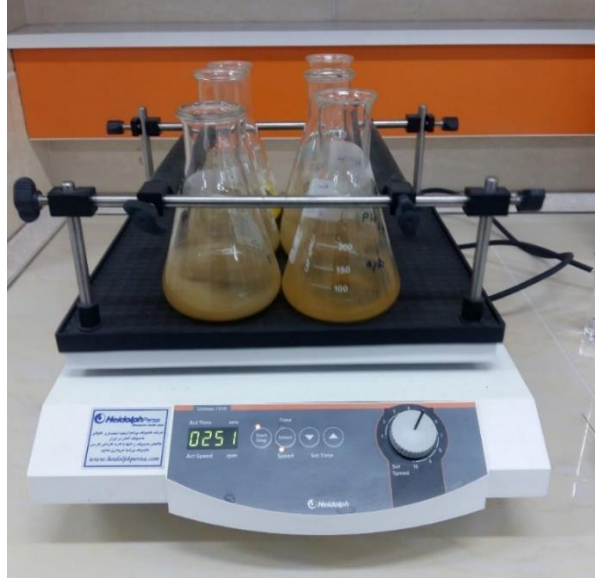
Fig. 34 Batch experiments using granular bentonite for the treatment of real textile wastewater (Laboratory of Water and Wastewater Treatment at Azad University in Iran)
