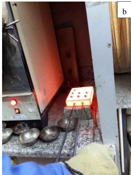
Fig. 38 (a, b) Thermal treatment of green granules in a muffle furnace (quality control laboratory at LECA CO.) (photo: E. Khalilzadeh Shirazi)
