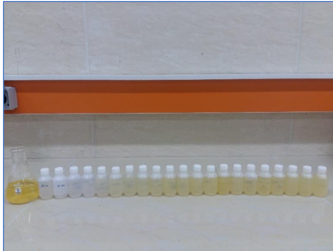
Fig. 79 Treated real acrylic fiber dyeing wastewater using fixed-bed column (Laboratory of Water and Wastewater Treatment at Azad University in Iran)
