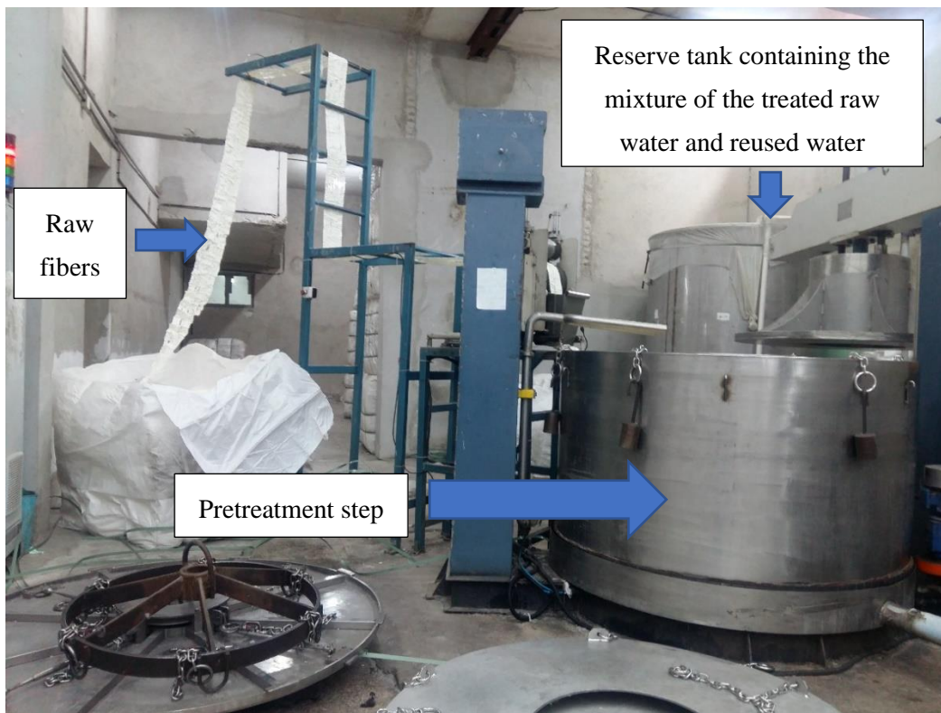
Fig. 80 Pretreatment of the fibers in the Acryl Tab CO.
