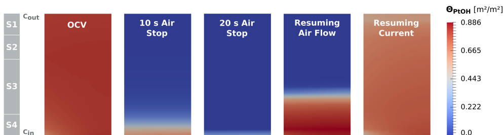
Figure 8.22: Catalyst surface coverage with PtOH in the CCL at different stages of the refresh cycle simulated with the transient DMFC model. The 2D plot shows the CCL magnified by 10^4 in x-direction.
