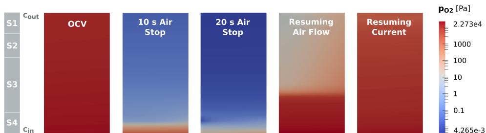
Figure 8.13: Oxygen partial pressure p_{\text{O}_2} within the CCL at different stages of the refresh cycle simulated with the transient DMFC model. The 2D plot shows the CCL magnified in x-direction by 10^4 and p_{\text{O}_2} on a logarithmic scale.
