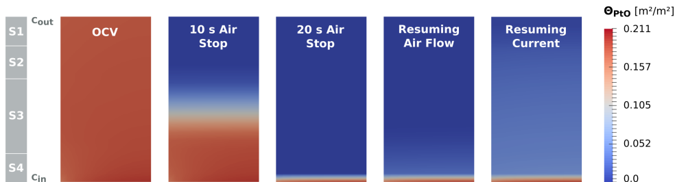
Figure 8.23: Catalyst surface coverage with PtO in the CCL at different stages of the refresh cycle simulated with the transient DMFC model. The 2D plot shows the CCL by 10^4 magnified in x-direction.
