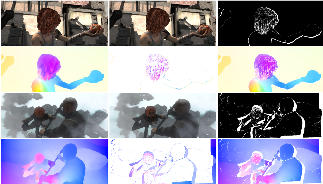
Figure 2.2: Examples of the Sintel dataset, occlusion map, and ground truth flow fields. Image source:[BWSB12]. The first two rows are an example of Sintel’s clean pass. From left to right, on the upper row are the first and second input images as well as the occlusion map. On the lower row are the ground truth flow fields of all pixels, occluded and non-occluded pixels. The last two rows are an example of Sintel’s final pass listed in the same order,
