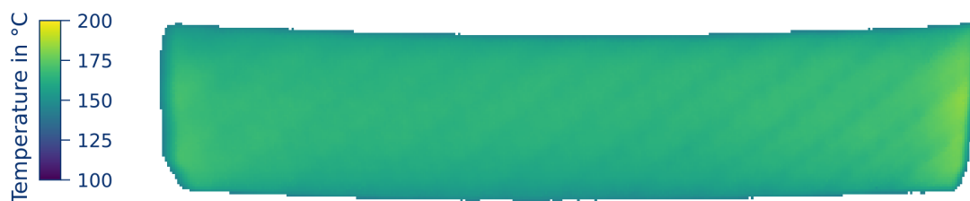
Figure 4. Temperature distribution of a prepregs heated for 10 s at 16 A with 12 mm contact width, rounded electrodes, and 20 kN contact force.
