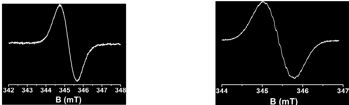
Figure 6.6.3. EPR spectra of electro-generated one-electron reduced species of 1^{\cdot-} (left) & 2^{\cdot-} (right) at 298 K in \text{CH}_2\text{Cl}_2 / 0.1 \text{ M Bu}_4\text{NPF}_6 solution.
