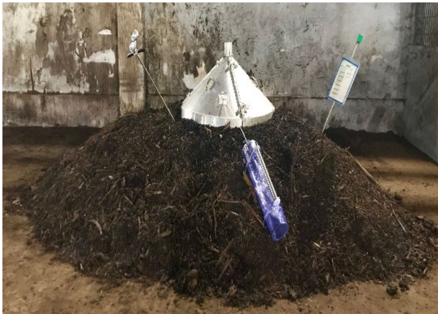
Figure 3 - 1: Gas measurement at the composting plant facility.
