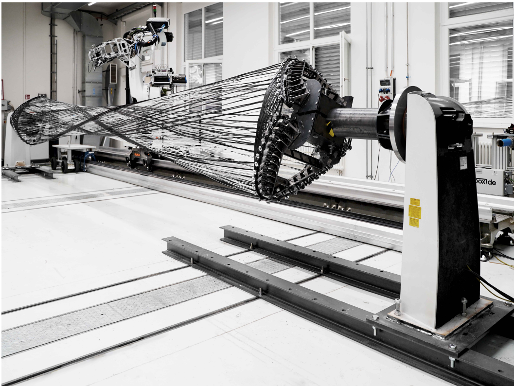
Figure 2.10: CPRCFW nine-axis kinematic system with 9-meter long component. ©ICD, University of Stuttgart.
