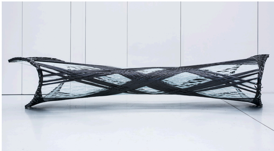
Fig. 11. RCFW demonstrator: G/CFRP composite element at 1:1 scale, (c) ICD.
