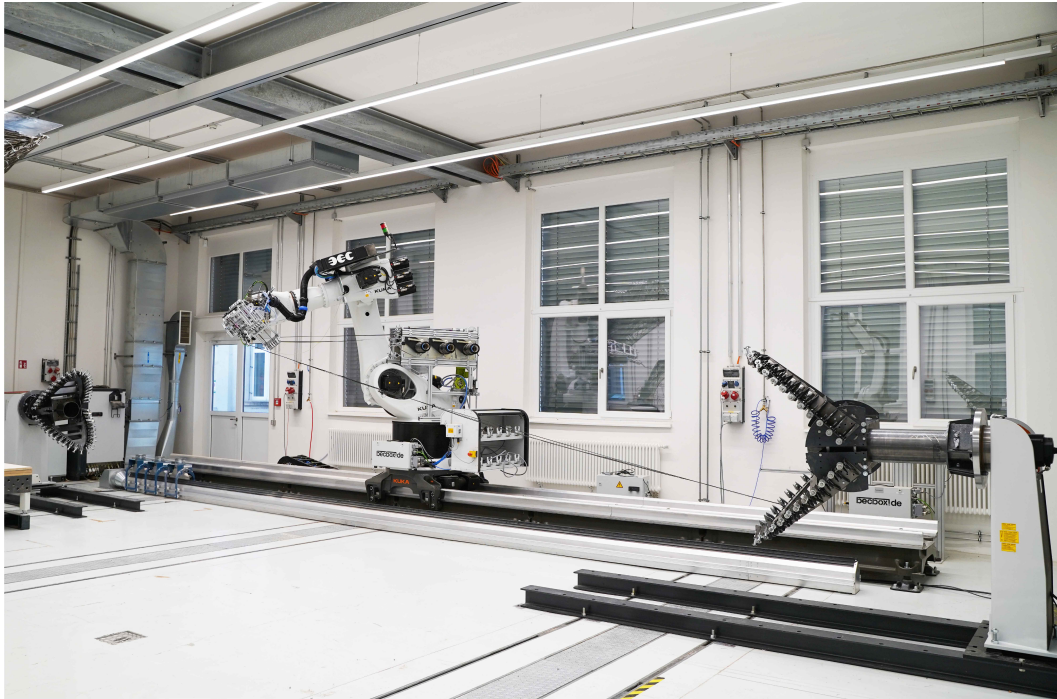
Figure 2.5: Steel winding scaffolds for industrial fabrication of the BUGA Fibre Pavilion by FibR GmbH. ©ICD, University of Stuttgart.
