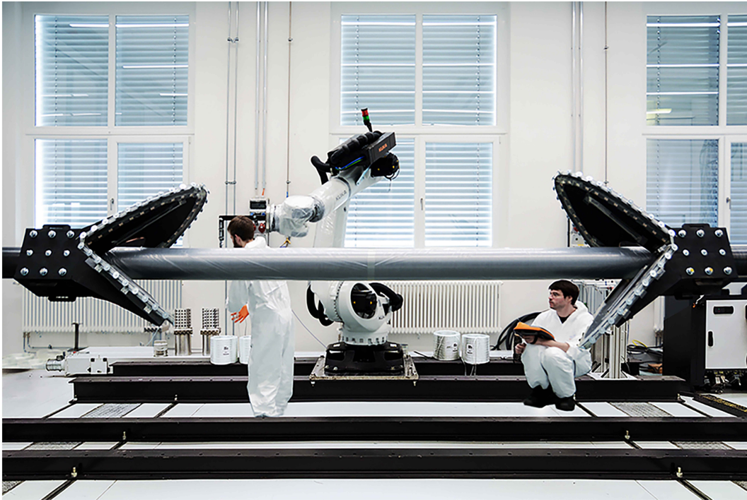
Figure 2.4: Timber winding scaffolds for research and development. ©ICD, University of Stuttgart.
