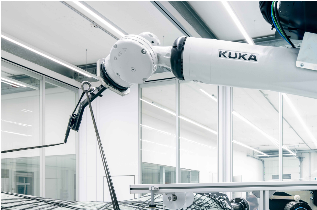
Figure 2.11: Single-purpose winding eye: fiber guiding. ©ICD, University of Stuttgart.
