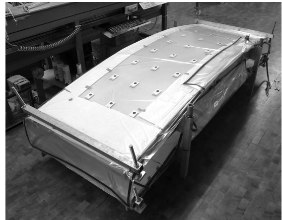
Figure 4.2.: Cold bending aluminium mould with glass-interlayer stacks wrapped in an evacuated vacuum bag applied in this research.
