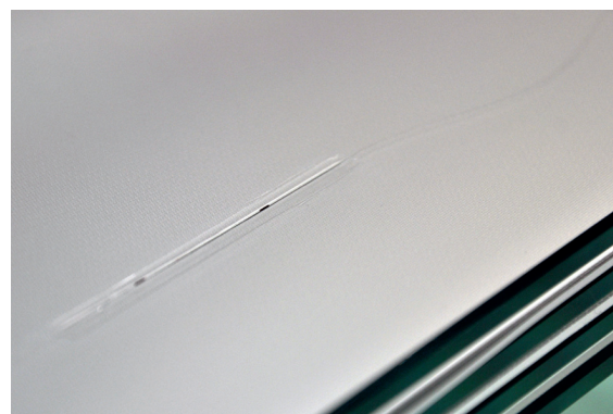
Figure 7.8.: Sensor glued to the interior glass surface of the four-ply laminate with Delo KB OB642.
