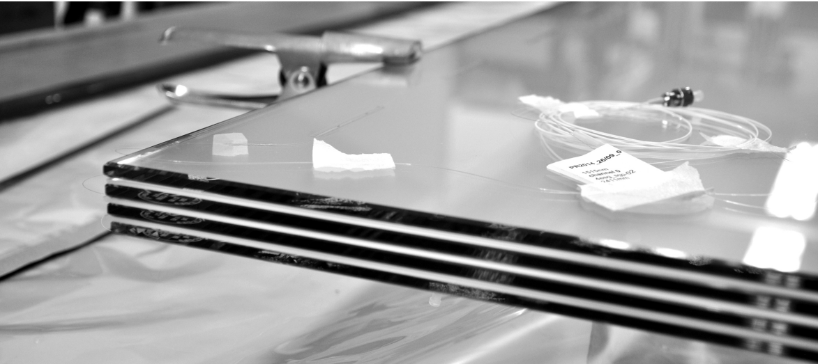
Figure 6.7.: Layout of sensors in the four-ply glass laminate prior to lamination.
