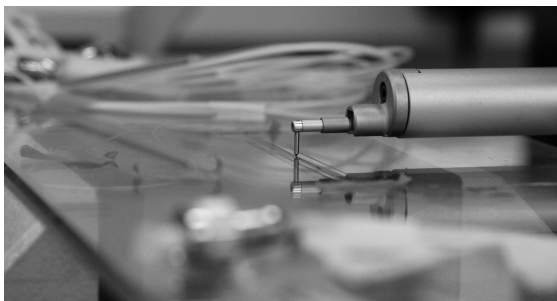
Figure 5.27.: Surface roughness contour measurement gauge head.
