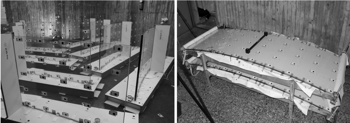
Figure 6.9.: Left: Setup of long-term testing of nine glass specimens; right: Photogrammetry setup at release of the glass samples from the bending mould.
