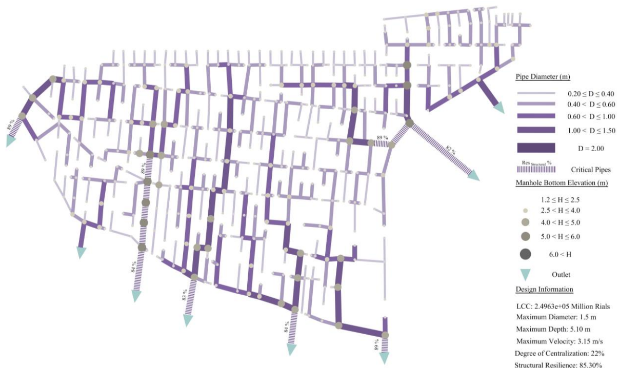
Figure 7. Design 1 (life cycle cost (LCC) = 249,630 M. Rials and degree of centralization (DC) = 22%).
