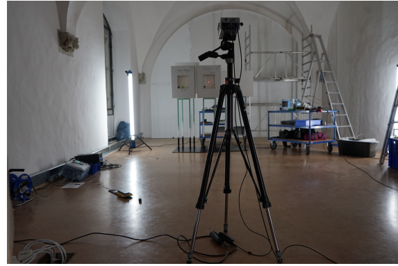
Fig. 2: Setup in the Renaissance Hall of ground measurements and vibration analysis on the hanging system with an accelerometer and Laser Doppler Vibrometry.
