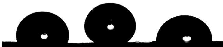
Figure 5.13 Contact angle measurements using a sessile drop of water. from left to right on: fresh AB35-GDE taken out of the press. after thermal treatment and spent GDE after electrolysis
