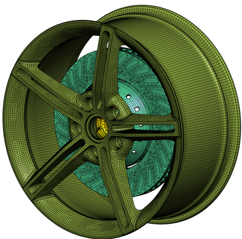
(a) Iso-view of the discretized assembly, consisting of the rim (green), a brake rotor (mint) and a wheel hub (yellow).
