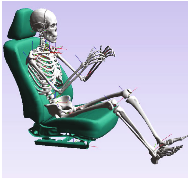
FIGURE 6 The skeleton of the EMMA4Drive manikin based on the THUMS Skeleton.
