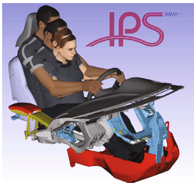
FIGURE 5 Simulation of a family of DHM sitting in a car holding the steering wheel.
