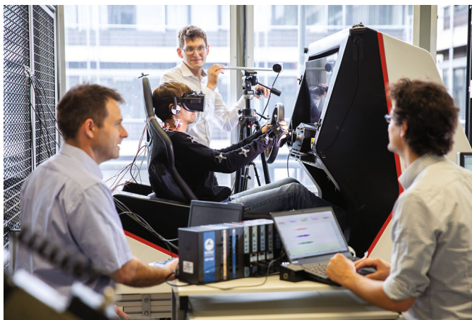
(A) Driver-in-the-Loop (DiL) simulator setup
