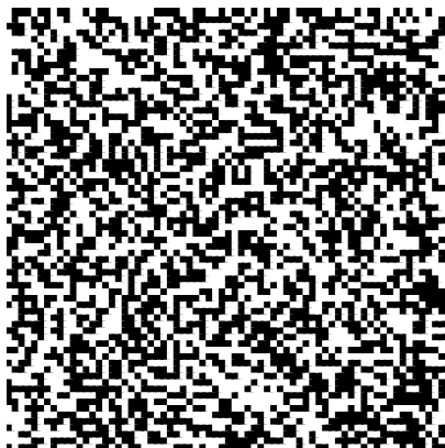
Figure 6.5: Binary image of the extracted random bits from |\Psi^-\rangle . In this binary image, no obvious patterns can be seen.
