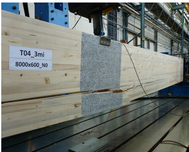
Figure 6. Tensile failure of T04.
