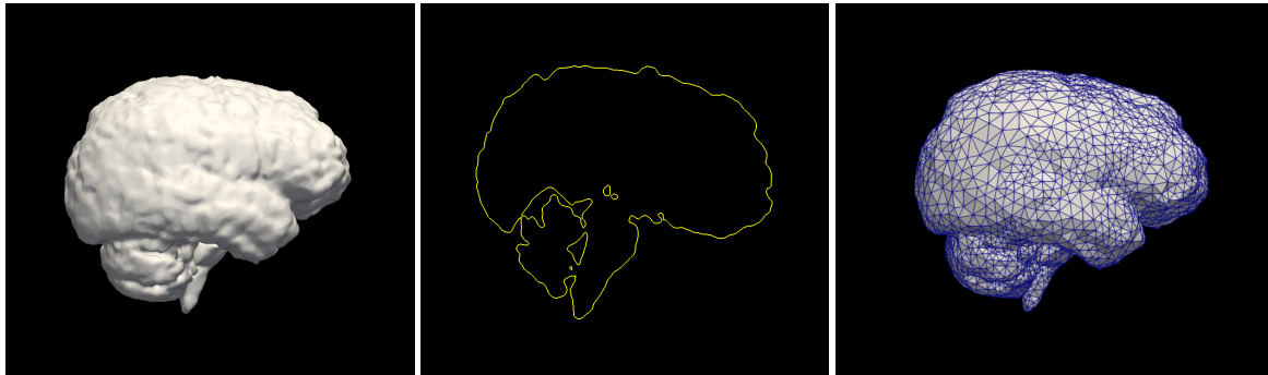
Fig. 3: Workflow of patient-specific data (subject 57, BraTS 2020) from NifTi 3D image (left) over watertight surface mesh (center) to processable volume mesh (right).
