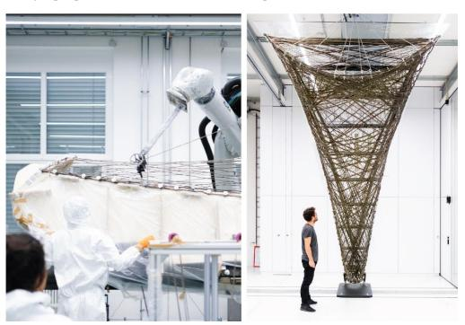
Figure 12. First full-scale prototype to provide feedback on fiber layup and material system.
