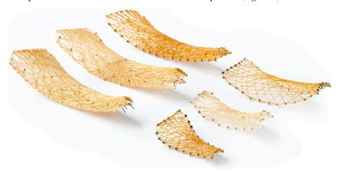
Figure 8. Different fiber patterns and anchor configurations to explore the component design space.
