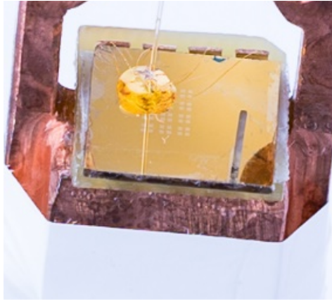
Figure 7.3: Picture of the first fiber-coupled detector design mounted on the previous sample holder and contacted with the four copper wires. One can clearly notice the optical fiber on top of the detector structure.
