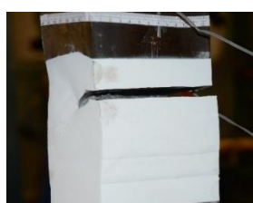
Figure 2: Butt weld with 80 mm thickness after failure [3].
