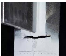
Figure 5: Crack at the end of a fatigue test with an attachment length of 500 mm [3].
