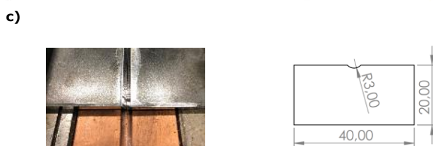
Figure 1 a) Verification measurement using a flat copper bar as backing with spatially resolved cooling time, b) temperature curves for TC-Type C and line measurement using an IR-camera with \epsilon = 0,8 , c) flat copper backing bar, d) angle copper backing bar, and e) ceramic backing bar
