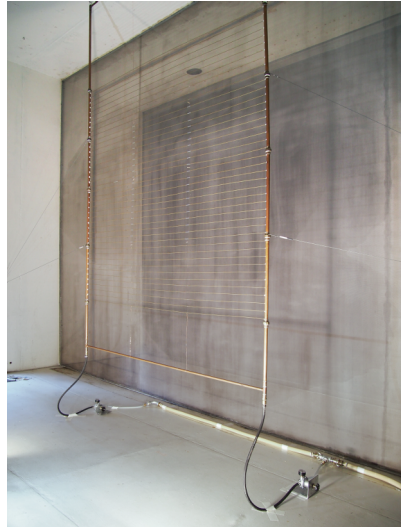
(b) Installation in the settling chamber.
