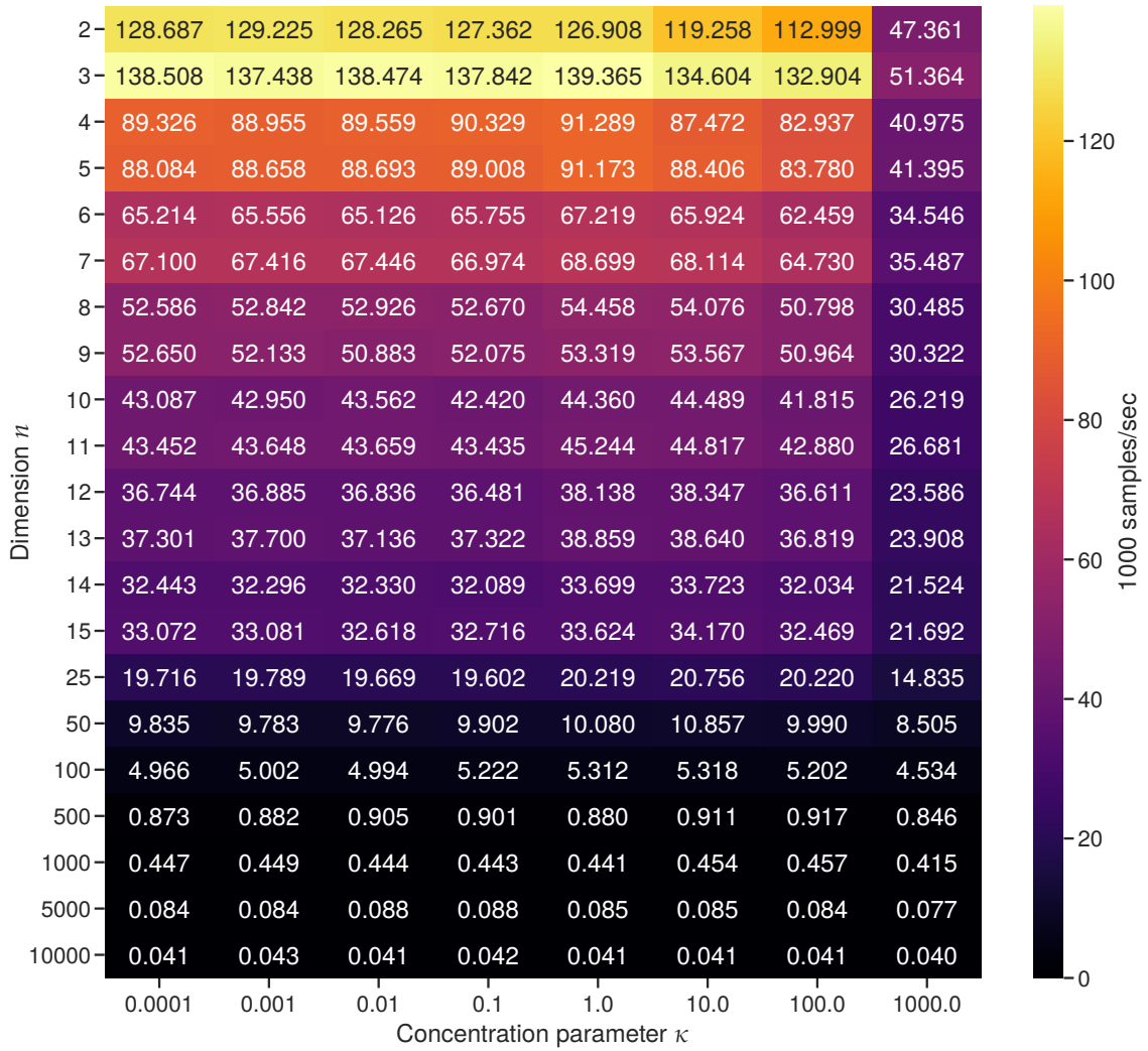
Figure 7.4: Sampling rates ( \times 10^3 ) of the Purkayastha approximate inversion method (Algorithm 3, vectorized implementation) with various parameters.
