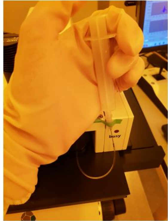
Figure 1.14 Photograph of injecting photoresist setup utilized for multi-responsive materials.
