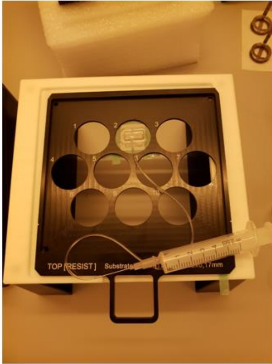
Figure 1.14 Photograph of injecting photoresist setup utilized for multi-responsive materials.
