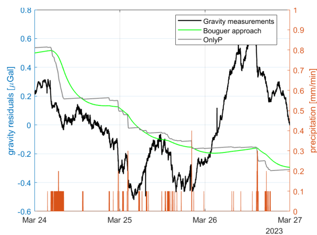
Figure 6.16.: Gravity responses of the two baseline models over the problematic March 24th event
