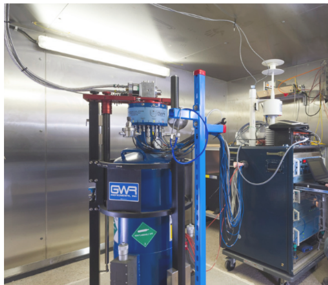
Figure 2.5.: The superconducting gravimeter of the BFO. The blue container on the left side is the Dewar. The silver cube on top is the cold head (Duffner et al., 2018)
