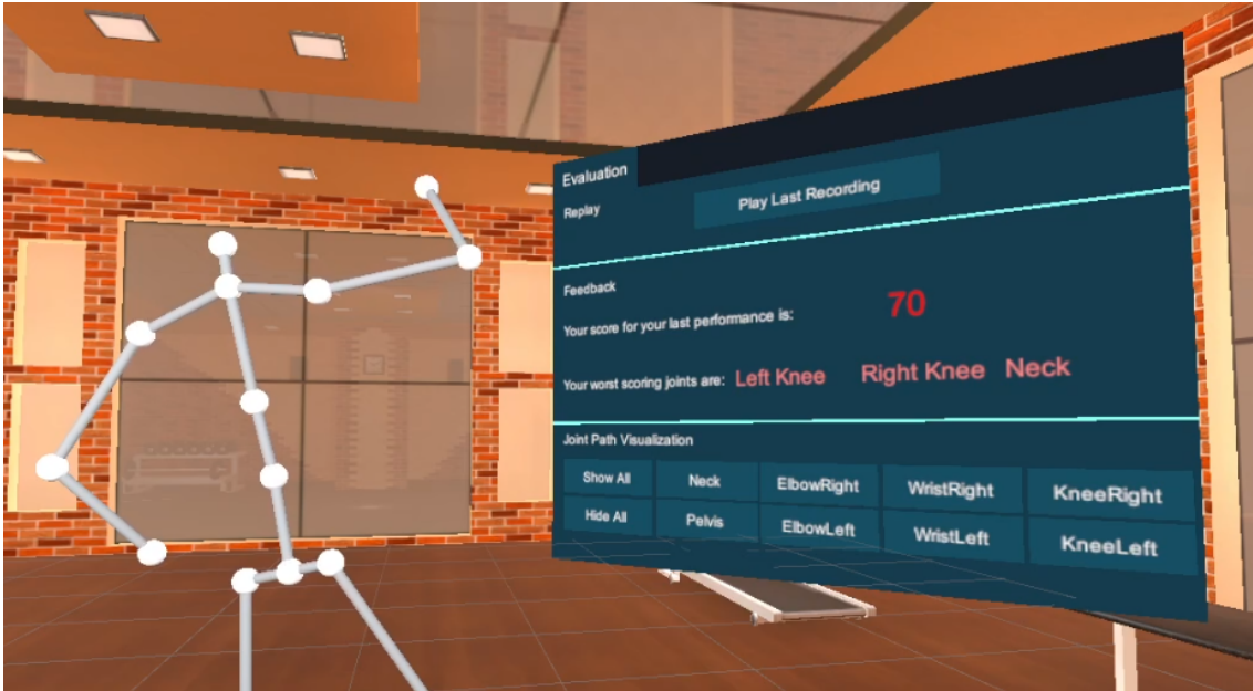
Figure 2.6: Example of abstract and natural feedback mechanisms taken from LiftVR. The white stick-and-balls skeleton is an instance of natural feedback, while the evaluation screen contains the abstract textual “score” and “worst performing joints” mechanisms.
