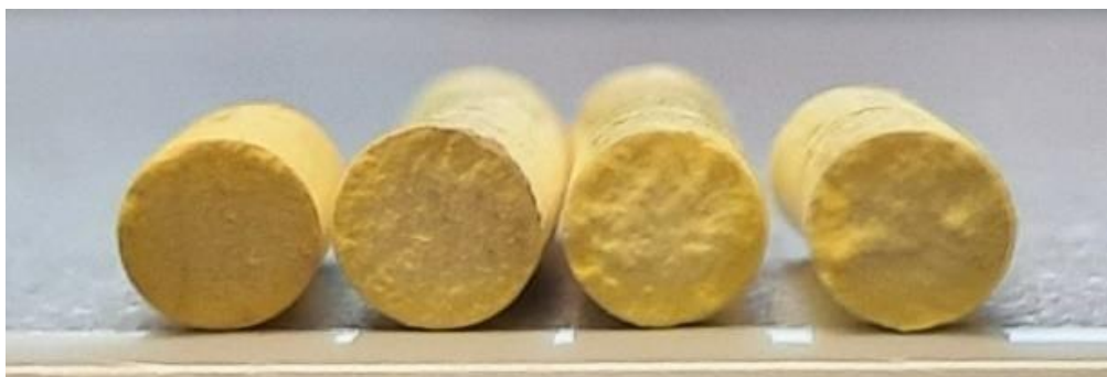
Figure 59: ROMP-derived monolith structure after hydrosilylation reactions.
