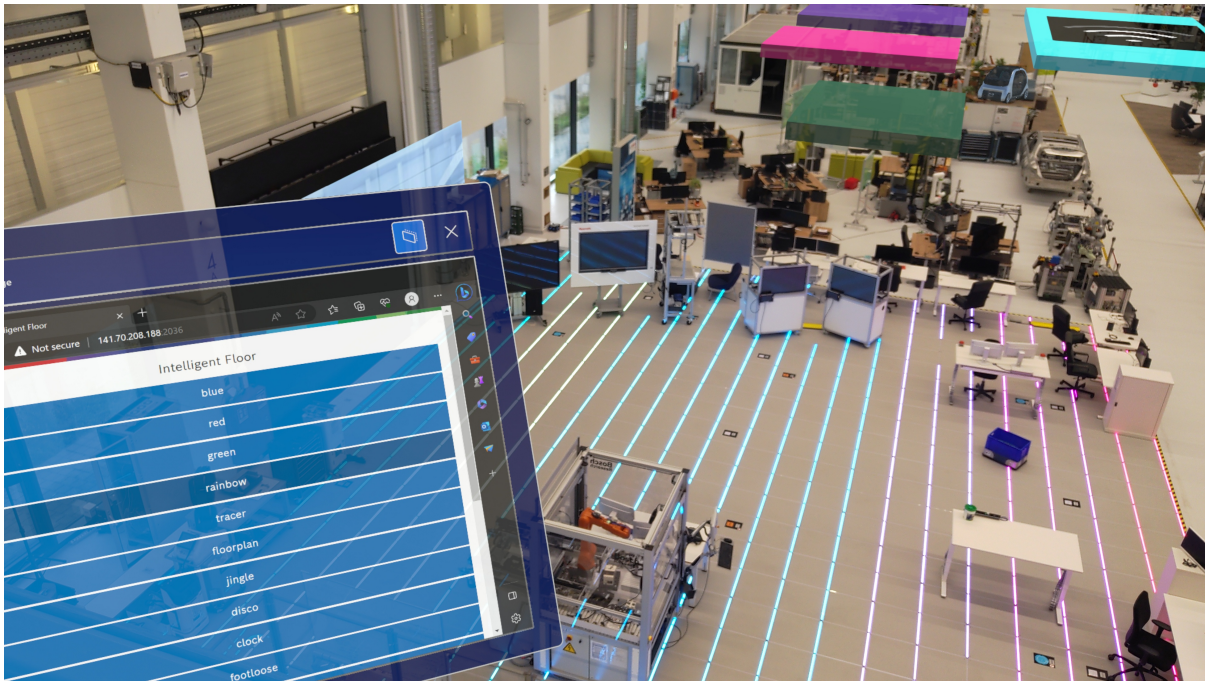
Figure 3.3: The Intelligent Floor being controlled via a 2D-interface. In this picture, the "rainbow" color effect is shown.
