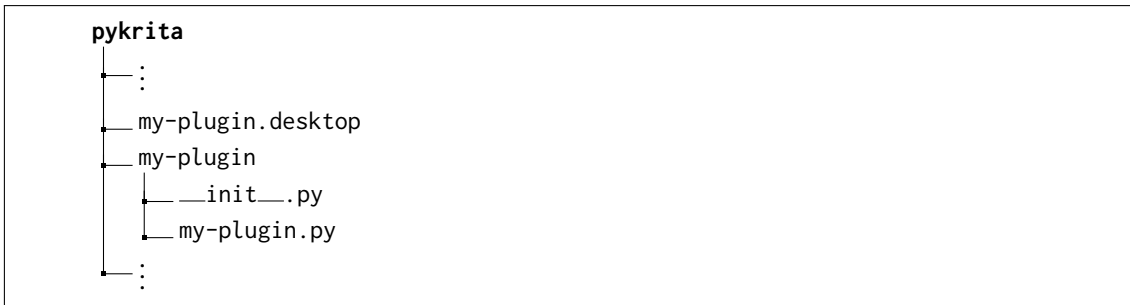
Figure 5.1: Plugin File Structure: The file structure how the sample plugin my-plugin is included into Krita. The plugin can then be enabled in the settings of the painting program.
