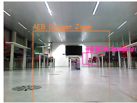
(f) The AEB ADAS recognizes the persons a few moments after they are removed (in the distance is the third obstacle [Hun12], cropped)
