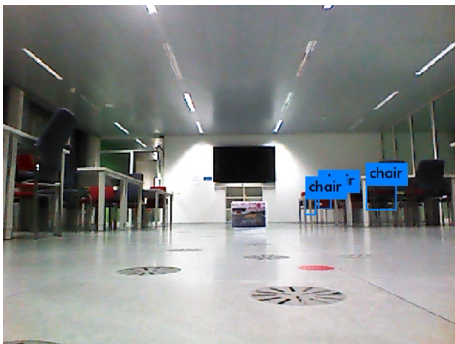
(c) The object detector recognizes multiple chairs (in the distance is the fifth obstacle [Kec13])
