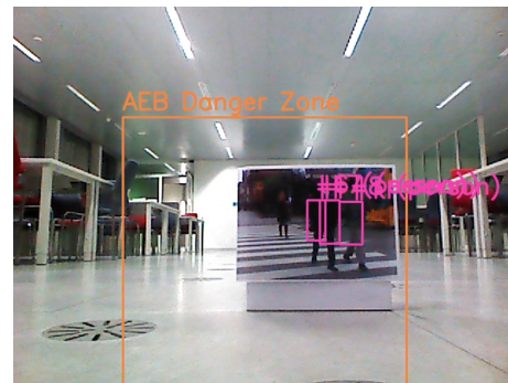
(d) The AEB ADAS recognizes the obstacle (multiple persons with multiple IDs) in the AEB danger zone (larger rectangle)
