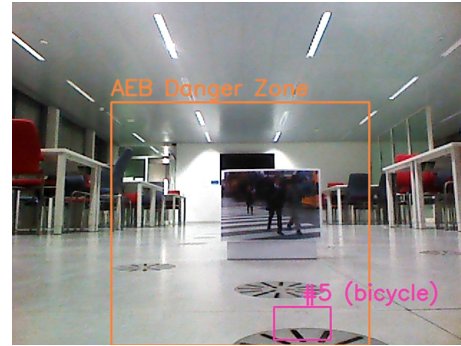
(b) The AEB ADAS processes the bicycle from Figure A.2a as object (ID #5) in the AEB danger zone (larger rectangle)
