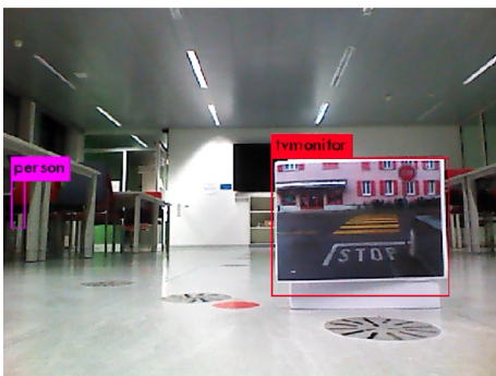
(c) The object detector recognizes a person and then the obstacle as tv monitor
