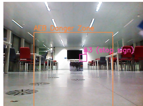
(d) The AEB ADAS recognizes the stop sign a few moments after it is removed (in the distance is the second obstacle [mal07])
