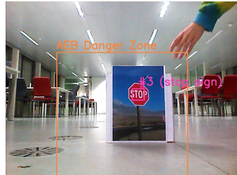
(b) The AEB ADAS detects stop sign (ID #3) in the AEB danger zone (larger rectangle)
