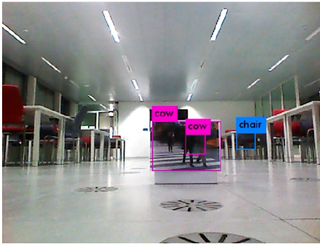
(a) The object detector recognizes the obstacle as cows as the obstacle is still far away. It also recognizes a chair
