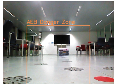
(d) The AEB ADAS does not recognize the objects from Figure A.5c, as they are not whitelisted
