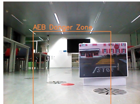
(d) The obstacle is not recognized as tv monitors are not whitelisted and the stop sign is outside the danger zone (rectangle)
