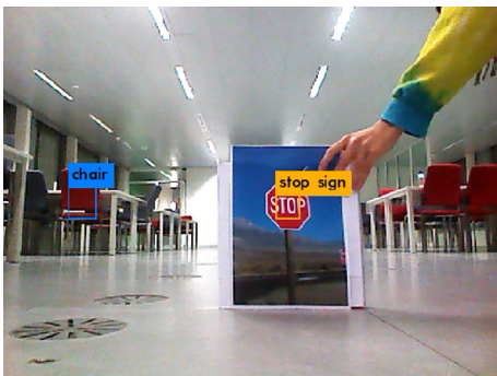
(c) The object detector recognizes a chair and the stop sign while AEB ADAS is cooling down the stop sign
