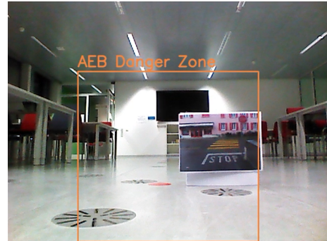
(b) As in Figure A.6a, the AEB ADAS does not recognize the obstacle
