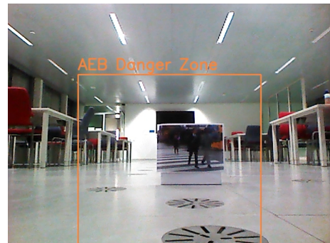
(b) The AEB ADAS recognizes no objects in the frame contrary to Figure A.2a
