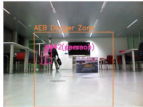
(b) The AEB ADAS recognizes the person multiple times as there are multiple bounding boxes and the person is moving (e.g., ID #42)
