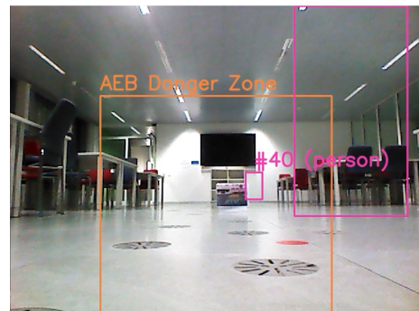
(d) Contrary to Figure A.4c, the AEB ADAS still recognizes the person, but with a different ID (ID #40) and the bounding box of the person that removed the obstacle (in the distance is the fifth obstacle [Kec13])
