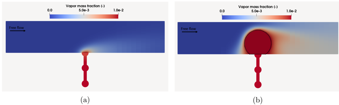
Figure 6.5: Distribution of vapor mass fraction: a) before droplet formation and b) after droplet formation.
