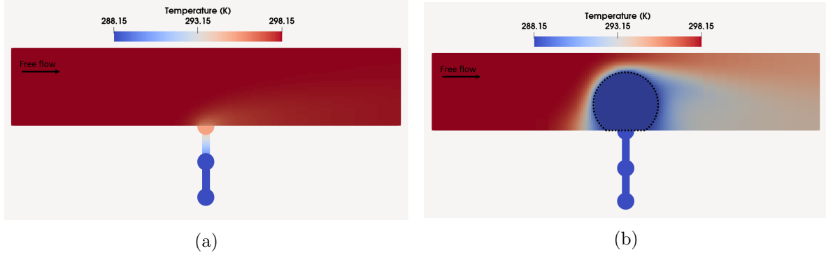
Figure 6.4: Temperature field: a) before droplet formation and b) after droplet formation.
