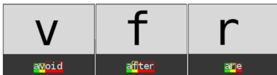
Figure 4.4: In GazeTheKey design, for each of the letters that will house word predictions, per key is estimated with previous letters entered by the user and letters associated with the key as input. In this image, the already entered letters to form words are in green, the letter on the key is yellow, and if the letter on the key is activated, then the predicted letters from the corpus to form the words are in red.
