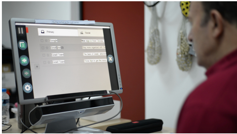
Figure 2.9: A photograph from Menges [110], showing MAMEM trials where participants suffering from Parkinson disease writing emails with the help of gaze input.
