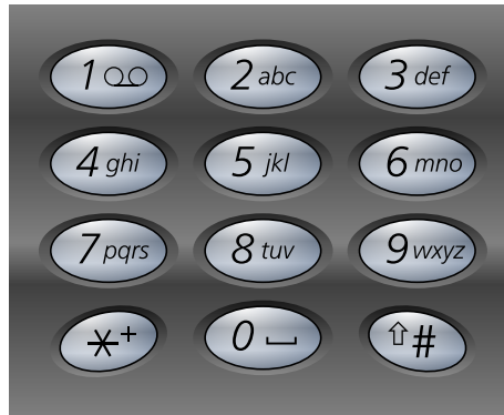
Figure 2.4: The multitap keyboard in the earlier generation mobile phones before the touchscreen era. Each key had 3 letters except number 7 and 9. The 0 was used for entering a space.
