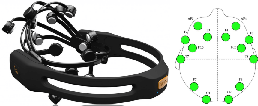
Figure 5.1: The image shows us the Emotiv EPOC+ headset with 14 electrode combination for capturing EEG data.
