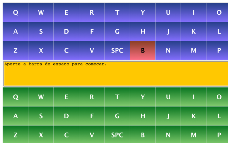
Figure 3.2: Context Switching Keyboard Design for saccade-based selection. The two separate regions of the keyboard (purple and green) represent two contexts. Focusing on the keys is done by short dwell times, and selection to type words is done by “changing” the context to the other keyboard and letter. Users can comfortably explore the whole content of a context without the effects of the Midas Touch problem.
