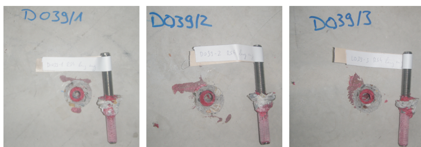
FIGURE B.102: D038 - Failure of the anchors
