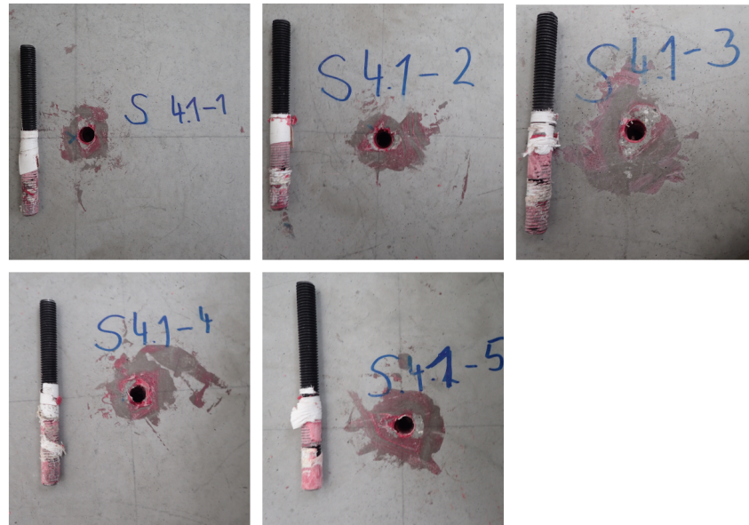
FIGURE C.95: S4.1-C - Failure of the anchors
