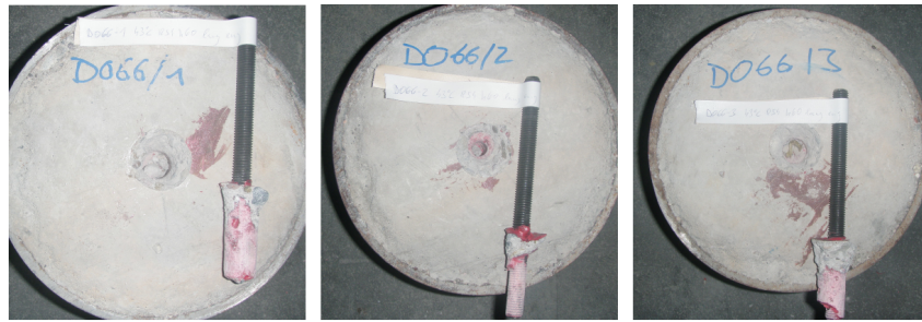
FIGURE B.114: D066 - Failure of the anchors
