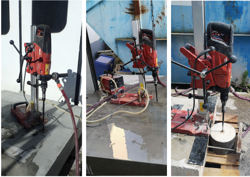
FIGURE A.2: Diamond core drilling system
