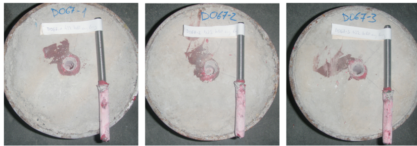
FIGURE B.114: D066 - Failure of the anchors
