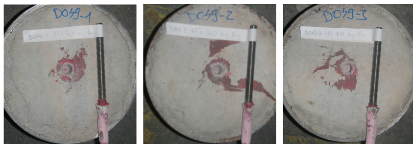
FIGURE B.110: D049 - Failure of the anchors
