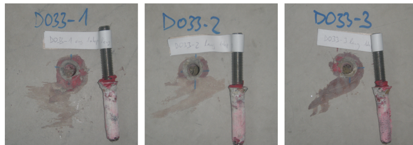
FIGURE B.99: D033 - Failure of the anchors
