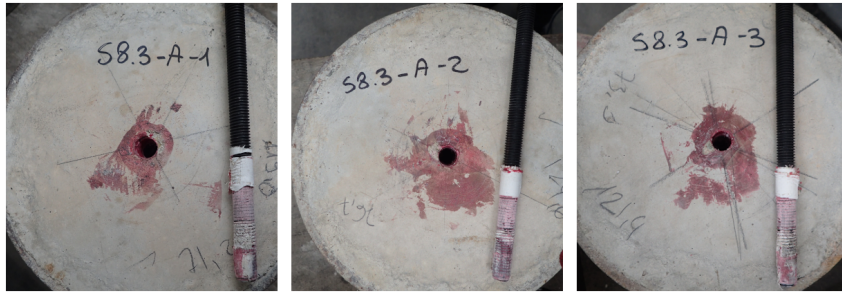
FIGURE C.126: S8.3-A - Failure of the anchors
