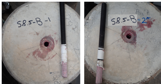
FIGURE C.128: S8.5-B - Failure of the anchors
