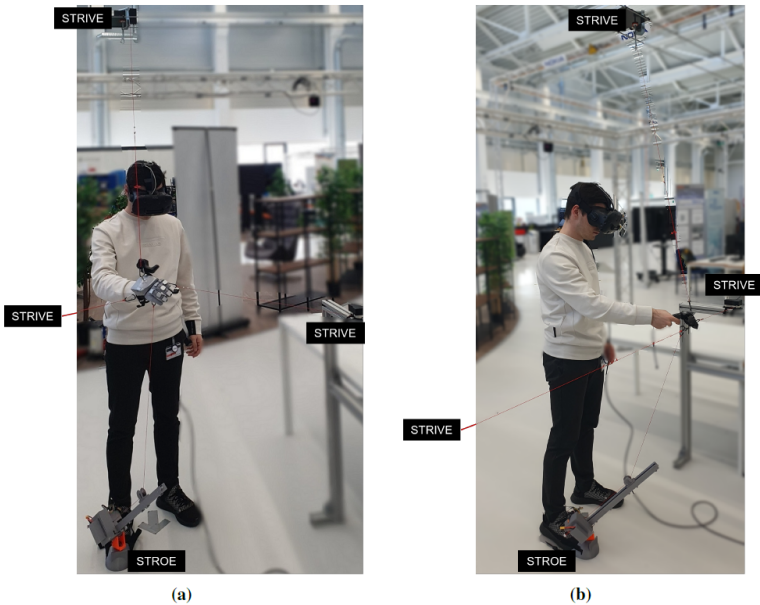
Figure 6.3 — Left: The study setup with SenseGlove, STROE and STRIVE. Right: The study setup with a HTC Vive Controller, STROE and STRIVE.
