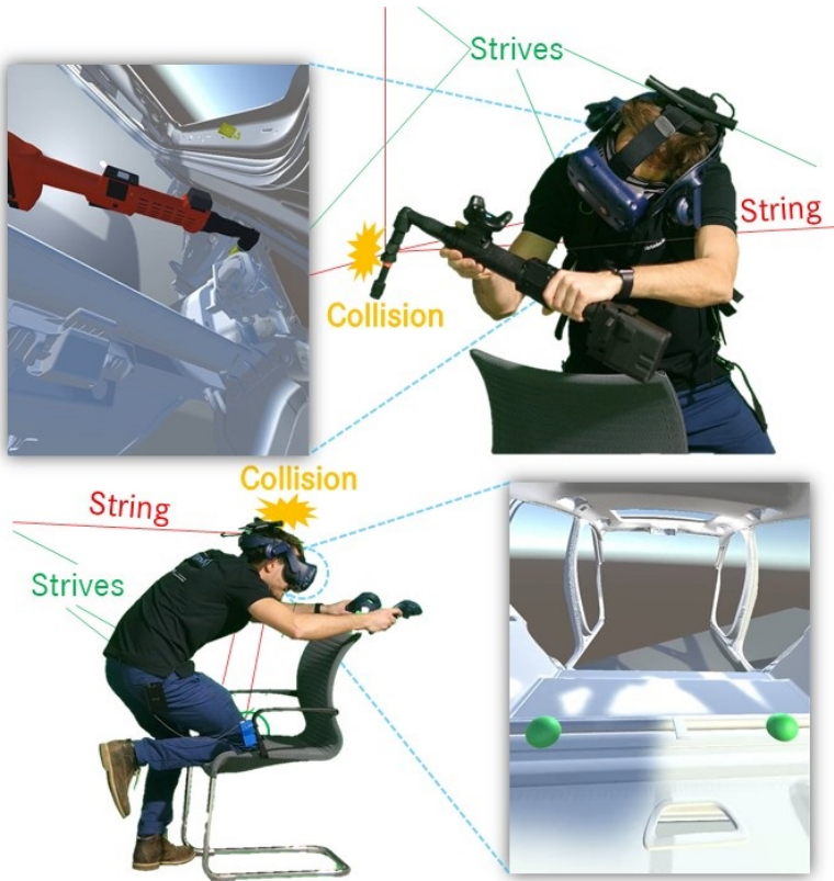
Figure 4.1 — The use of STRIVEs in two automotive use cases. On the left, an assembly task in a trunk in which STRIVEs provide force feedback on the user’s head. On the right, a screwdriver task in which the user feels forces acting on the screwdriver. Most of the STRIVEs boxes are not visible in this figure because they were mounted outside the picture.
