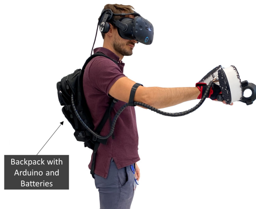
Figure 3.1 — Left: PropellerHand consists of two propellers in rotatable cages attached to a glove. Right: A user wearing the device. The control unit and batteries are placed in a backpack to reduce the weight of the hand-mounted hardware.
