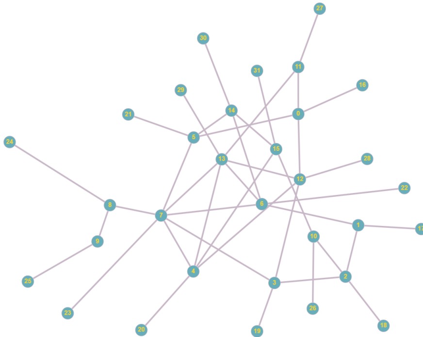
Figure 6.2: The medium-sized topology used for empirical testing with 16 devices and 16 switches. Nodes numbered 0-15 are the switches and nodes numbered 16-31 are the devices.
