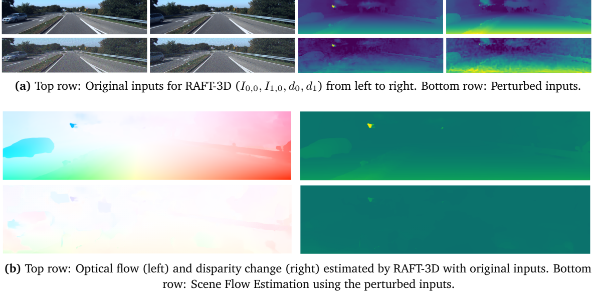
Figure 5.1: Experiment 37: The perturbation penalty terms use the factors \alpha = 500 and \beta = 20 . The perturbations of the disparities are more perceptible than the image perturbations. These perturbations lead to a scene flow estimation close to the target flow s_0 .
