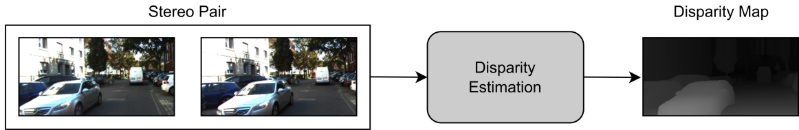
Figure 2.3: A disparity map encodes the disparity value for each pixel of the rectified stereo image pair.
