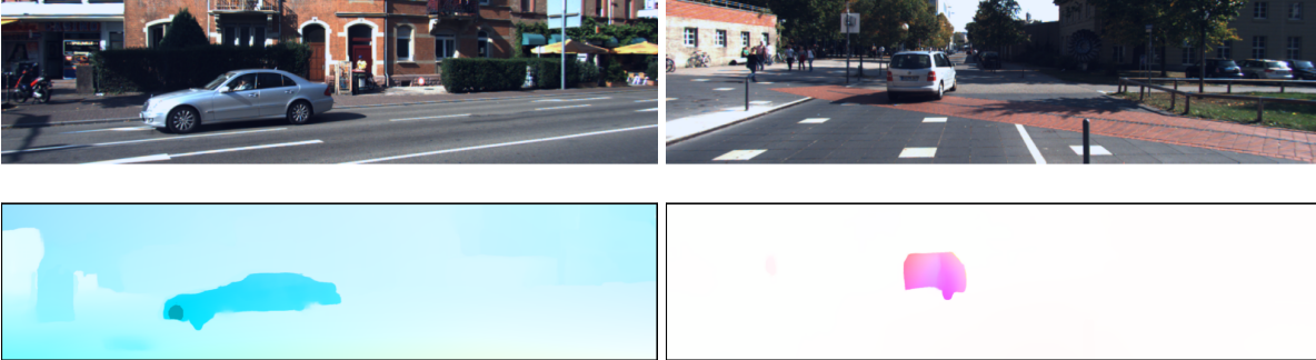
Figure 5.6: RAFT-3D is relatively robust against GSFAC-strict on particular KITTI scenes with high-contrast moving objects. Top: I_{0,0} of scene. Bottom: Attacked flow s^* .
