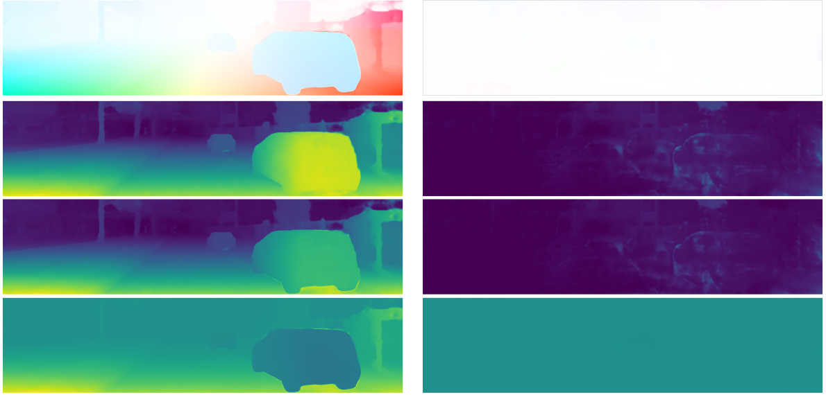
Figure 5.12: Left: RAFT-3D scene flow estimation (u, v), d, d', \Delta d from top to bottom. Right: Adversarial scene flow s^* after GSFAC-coupled.
