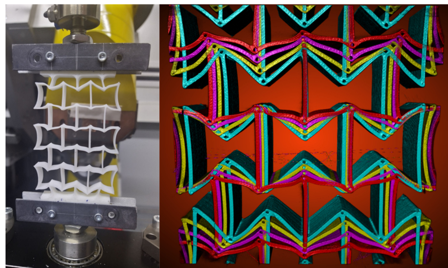
Figure 20. Deformed state of a 3 \times 3 PBAT sample (left) and the overlapping view of the sample at loading state of 0 mm, 5 mm, 10 mm, and 15 mm presented with cyan, yellow, magenta, and red color, respectively (right).
