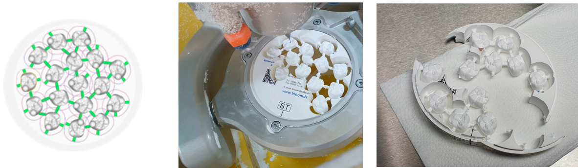
Figure 1. CAD/CAM preparation of zirconia crowns.
