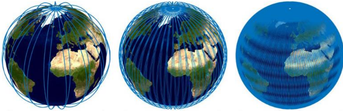
Figure 2.2: The path that the GRACE satellite mission follows is shown in three different time periods: one day (left panel), one week (middle panel), and one month (right panel). (credit: Szabó and Marjańska, 2020)
