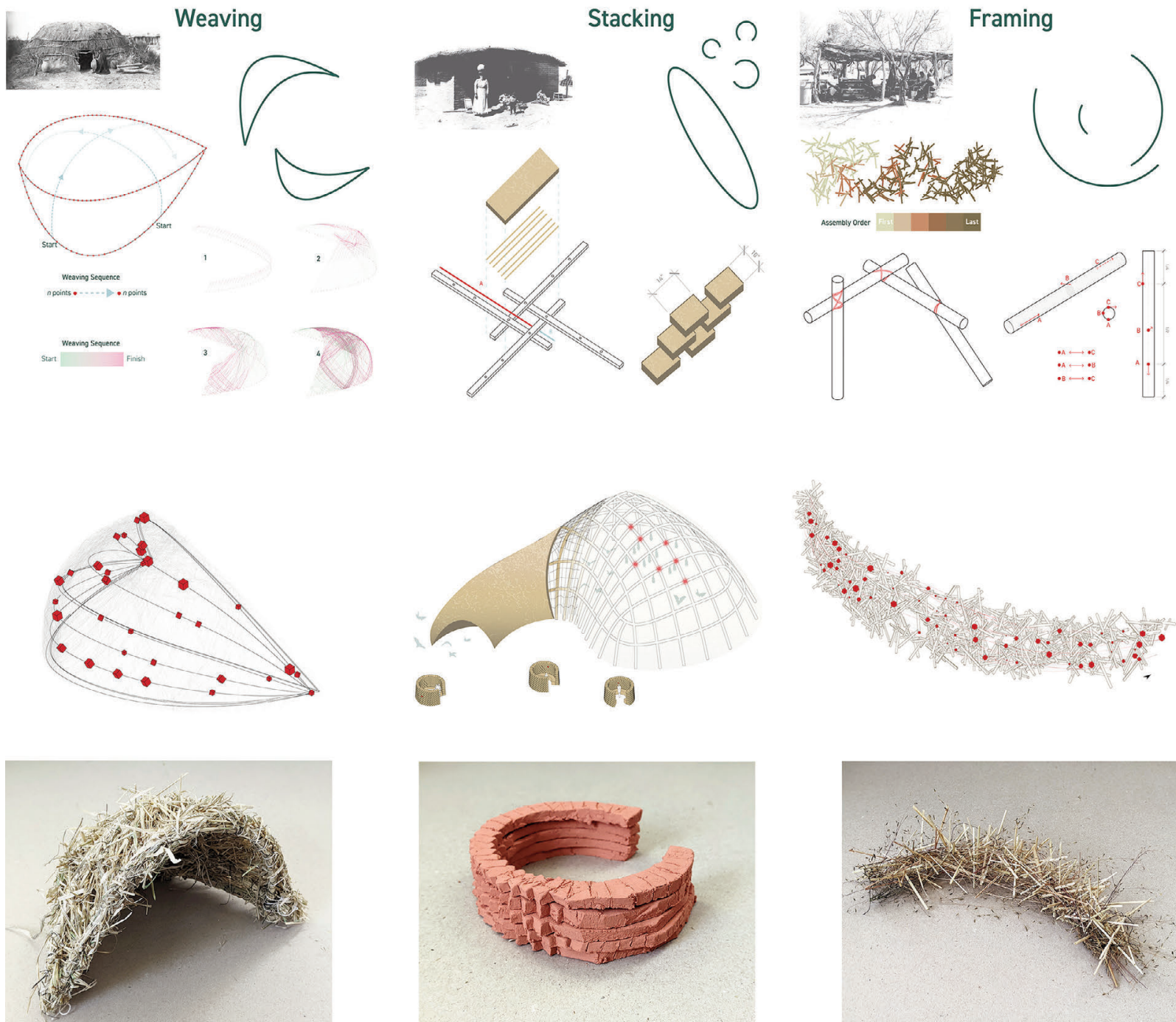
Fig. 14 | Proposed sites and methods for constructing prototypes based on weaving, stacking and framing (credit: C. Becerril and G. Veitch, 2022).
