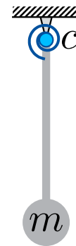
Figure 2.5.: Stiff pendulum with massless rod and point mass at the end, having one DoF, rotating around the joint (light blue) and connected with a torsional spring (dark blue) to fixed point in space.
