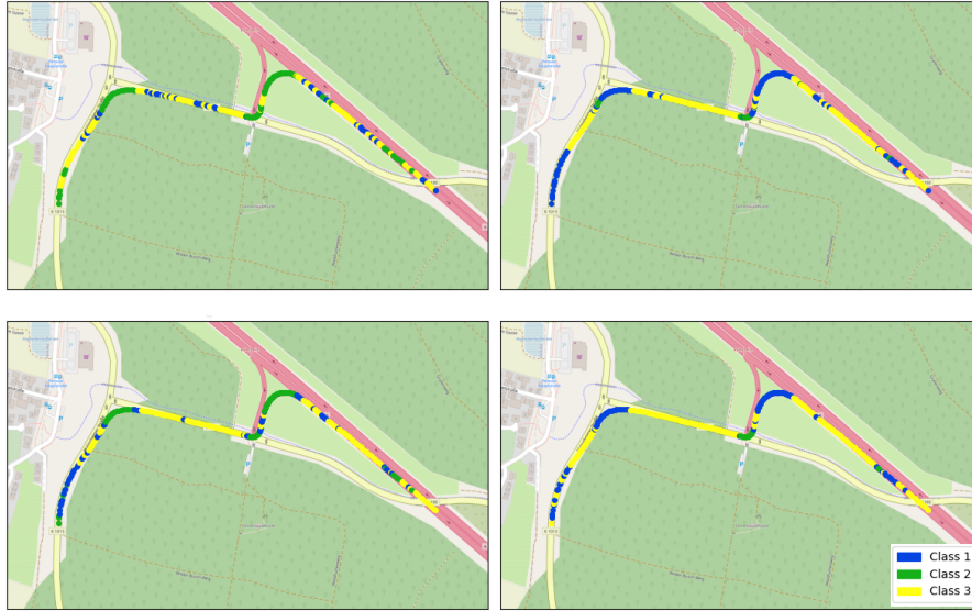
Figure 6.3: GPS visualization of clusters identified using DAE models for a Highway scenario. (a) Top left: Cluster outputs for DAE BN1 model with IPL 1.0s and LSD 9, (b) Top right: Cluster outputs for DAE BN1 model with IPL 1.6s and LSD 10, (c) Bottom Right: Cluster outputs for DAE BN1 model with IPL 1.0s and LSD 6, (d) Bottom Left: Cluster outputs for DAE BN1 model with IPL 1.6s and LSD 5.
