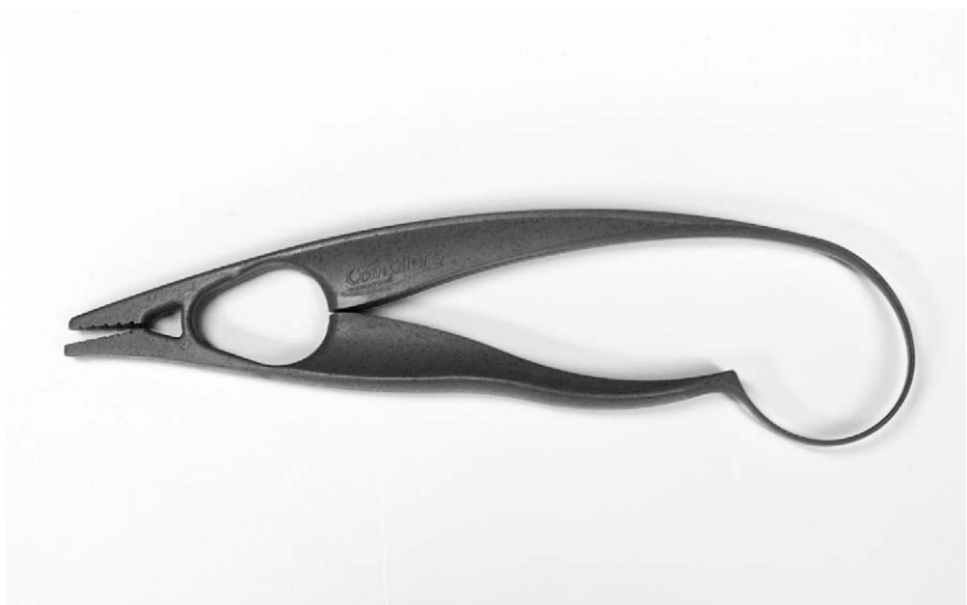
Figure 2.19: This fish hook remover is an example for a one-piece compliant mechanism. It features a deltoid Q-joint with a passive joint where the handles get into contact.
