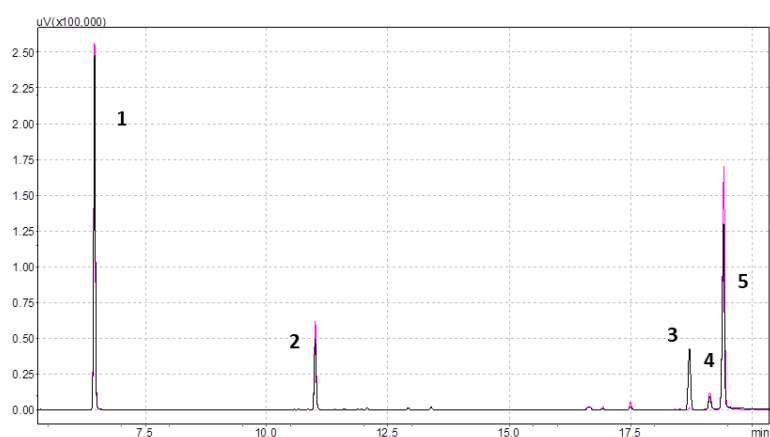
Fig. 4.3: GC-FID chromatograms of the conversion of homofarnesol with ZmoSHC1 (black) and negative control (pink), (1): internal standard 1 (ISTD1 1-decanol); (2): internal standard 2 (ISTD2 1-dodecanol); (3): product ambroxan; (4): ( E,Z )-homofarnesol; (5): substrate ( E,E )-homofarnesol.
